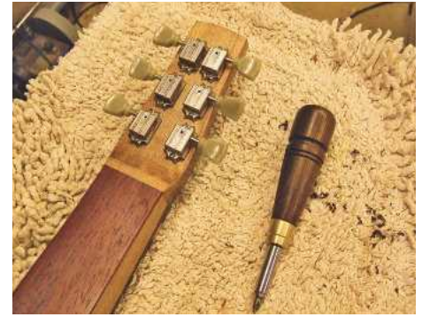
▲ Pic.29 Pre-drill the holes before screwing the tuners in position
